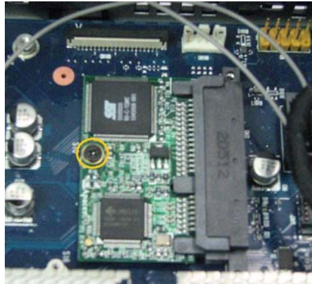
Figure 11 Removing the existing flash module
